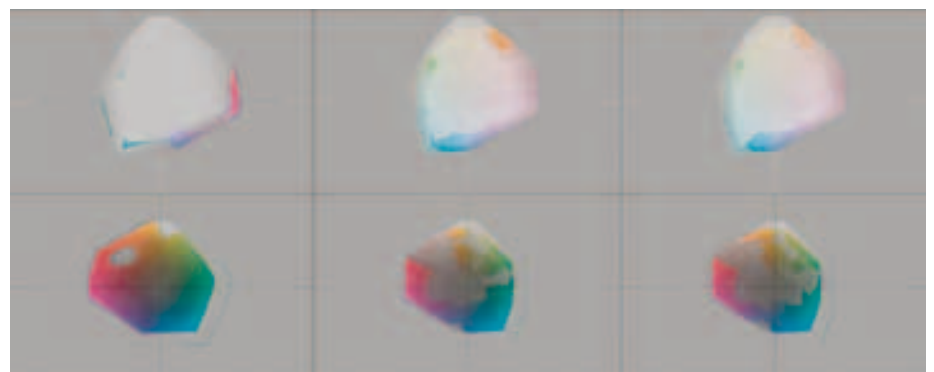
Top and bottom views of the shrinking newsink-newsprint gamut after 2 minutes, 4 hours and 24 hours. After 4 hours, the gamut has lost almost 15 % of its color. The grey areas show the gamut boundary of the ICC ISOnewspaper26v4 profile. The freshly printed color gamut retracts to a size even smaller than the de facto standard newsprint color gamut in this example.
