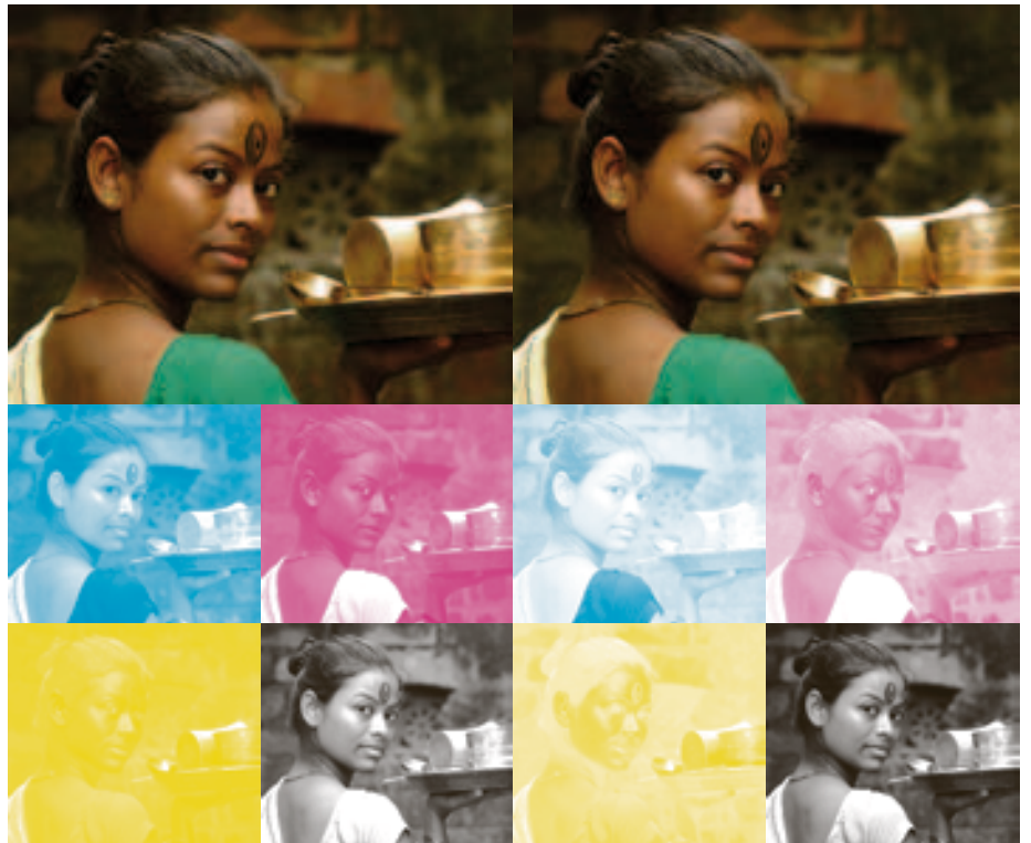
With GCR, the grey components of the chromatic color overprints are compensated by black, without this changing the color impression of the image. The image and separations on the left were produced without GCR, those on the right using GCR. The resulting savings can be considerable.
